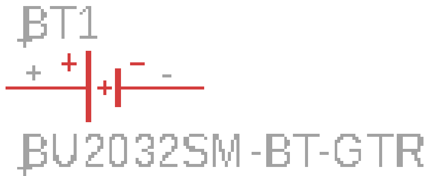
Figure 5-19: Schematic of BU2032SM Battery Holder
